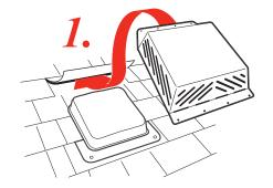
Place the VENTGUARD PLUS over the homes' existing roof vent and nail or screw down.
