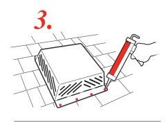
Seal all screw or nail heads with an outdoor sealant.
