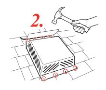
Use 2" screws or 2" roofing nails.
